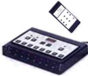
Fig. 2: “People Meter” Device for DTH type ROTs with Remote
